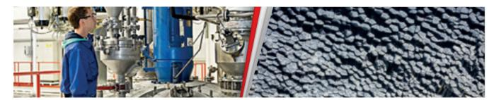
Sigmacure is the universal classic product: a Cold-Box binder system in which the two components, phenolic resin and polyisocyanate, come dissolved in aromatic solvents. This system provides foundries with a product line whose efficiency is based on decades of experience.
