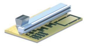
Conventional additives are not suitable for 3D printing due to their fine particles. The same applies to additives with a wide particle size distribution, which cannot be reliably applied using the recoater. Our AM additives are characterised by an optimal particle size distribution, which even at addition levels of up to 8%, does not result in a significant loss of strength for cores and moulds.
